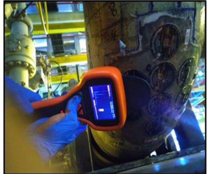
Testing for good signal after attaching the Sensors
