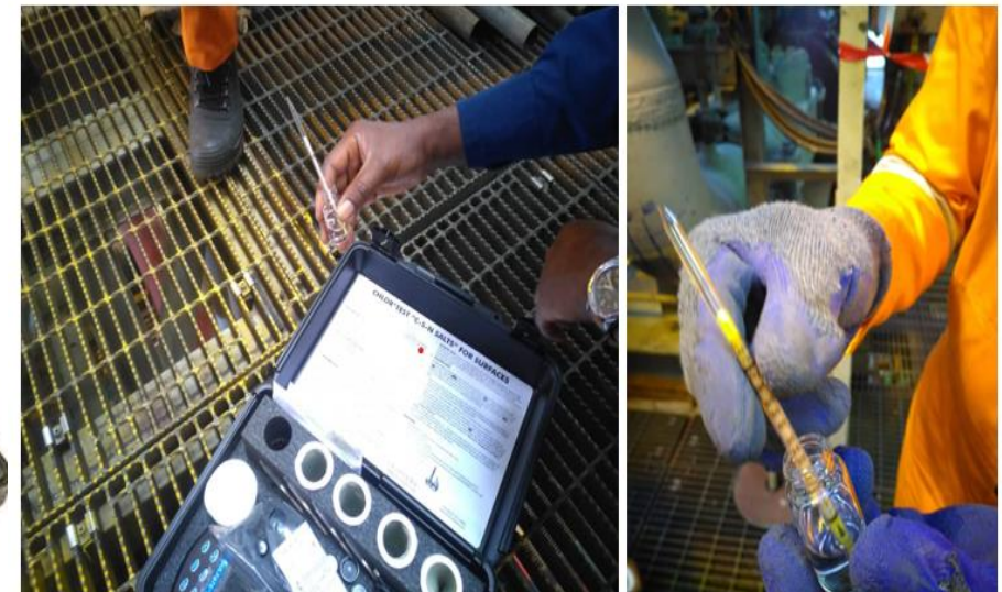
Conducting Chloride test
