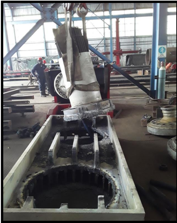
Tube sheet detached from the base support
