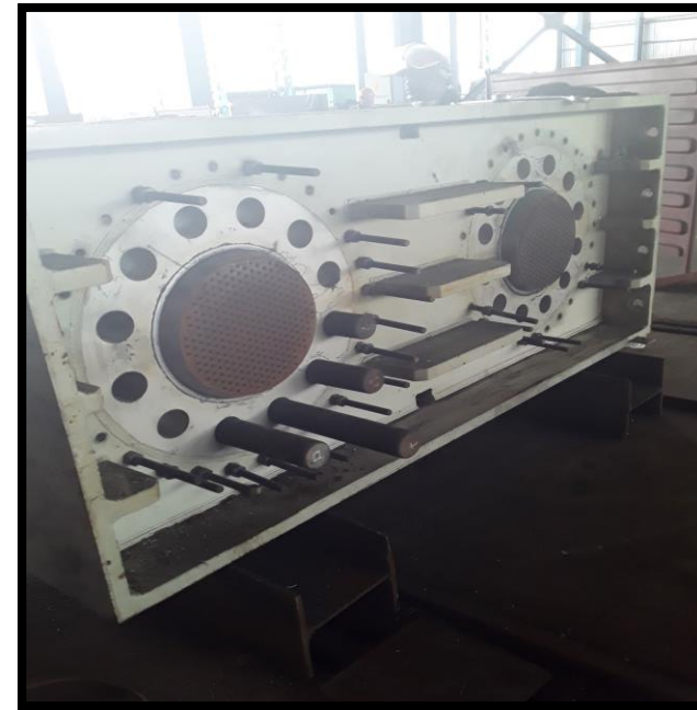
Exposed Tubesheet for Visual Inspection
